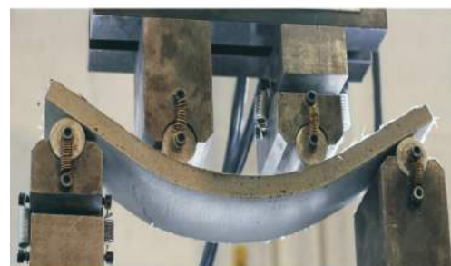
Toughness Test as per ASTM C-1018
