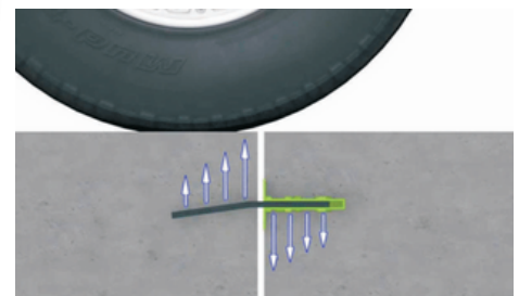
Load Transfer Mechanism
